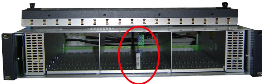
Figure 3-5 Front Panel-Close the Swivel Handle of the Module
