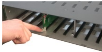
Figure 3-7 Press Down the Swivel Handle
