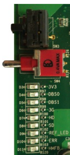
Figure 5-4 The Logo Printing of LED Indicator
