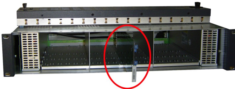
Figure 3-4 Front Panel-Push the Module into the Slot
