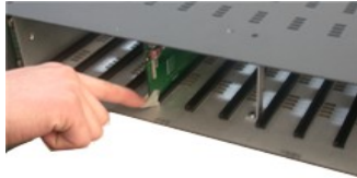
Figure 3-7 Press Down the Swivel Handle
