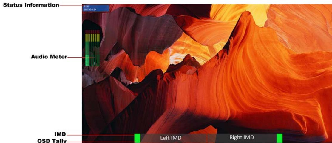
Figure 4-1 Features of LMW-550-4K Monitor
