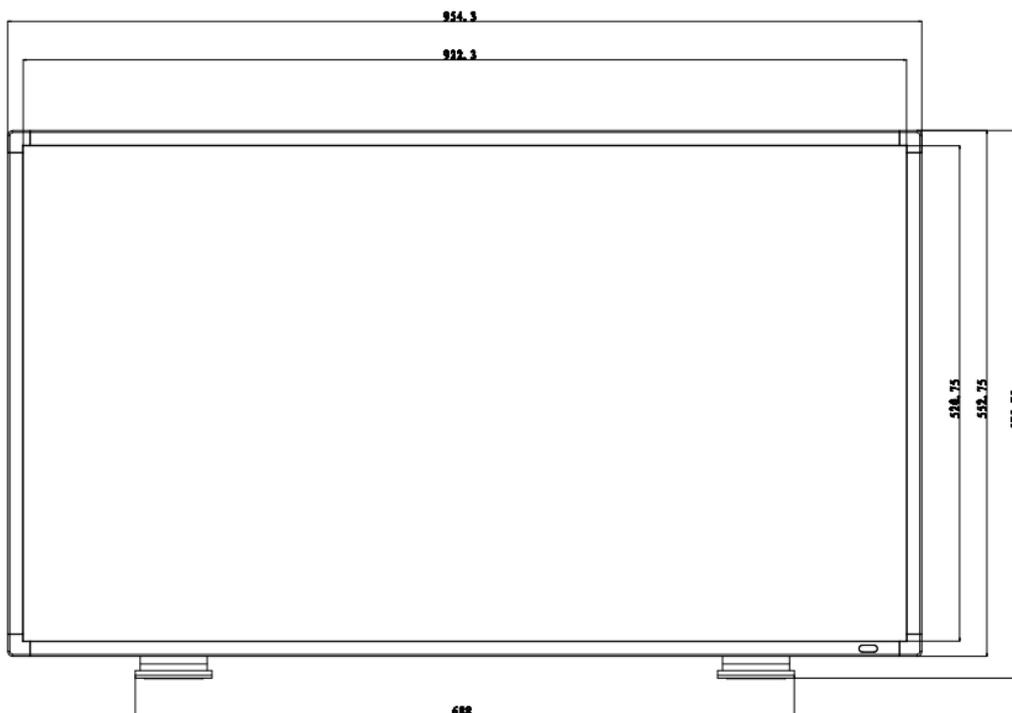
**Figure 7-1 Front Panel(Unit: mm)**
