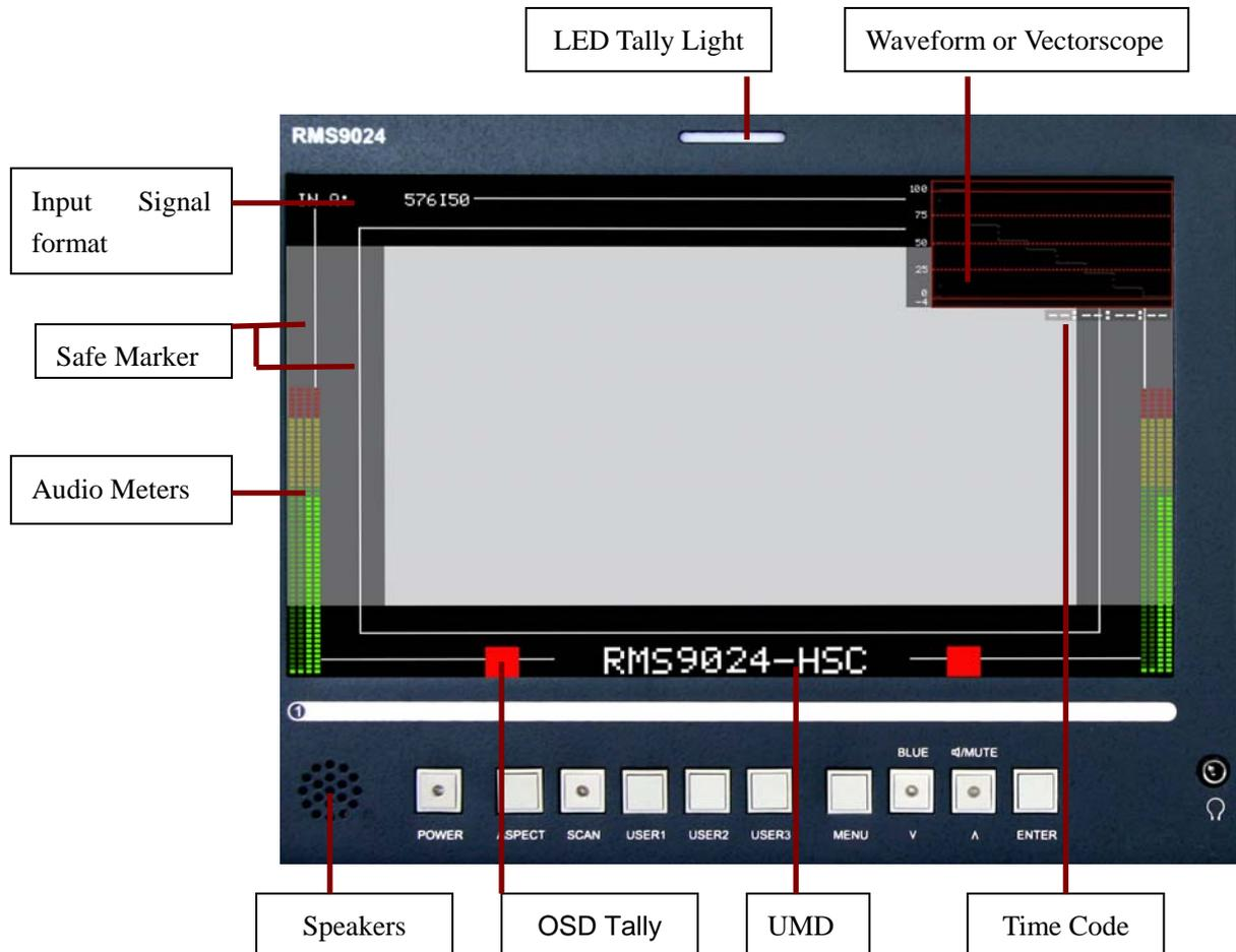
1. **LED Tally Light:** This tri-color (red/green/amber) light is controlled through a DB9 connector on the rear panel. For more information about the DB9 connector, refer to “Rear Panel” on Chapter 4.4.
